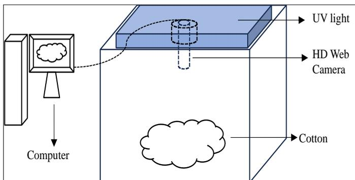
Figure 8. Prototype system design
