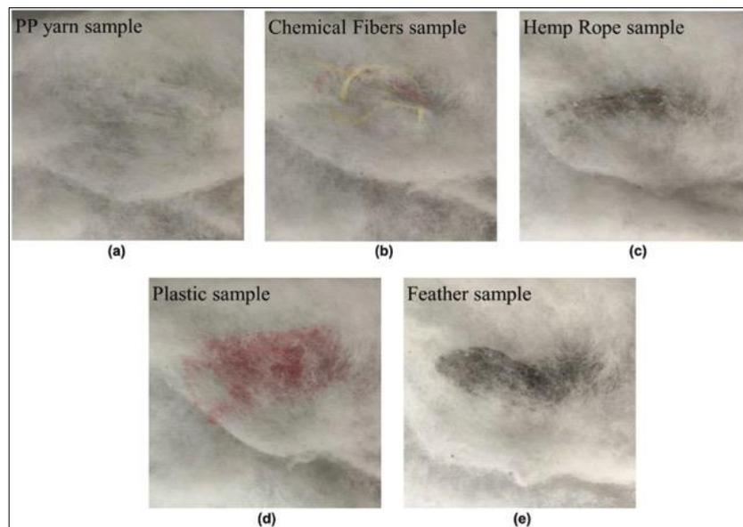
**Figure 1.** Foreign fibers experiment samples:(a) PP Yarn; (b) Chemical Fibers;(c) Hemp Rope; (d) Plastic; (e) Feather (Du et al., 2023)
