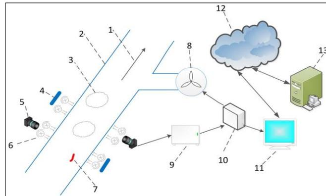
Figure 6. Structure diagram of foreign fiber cleaning machine. (1) Flow direction, (2) cotton pipe, (3) cotton, (4) background board, (5) the imaging unit, (6) tube, (7) foreign fiber, (8) removal fan, (9) processing subsystem, (10) classification subsystem, (11) industry personal computer, (12) Internet, and (13) cloud server. (Wei et al. 2019)
