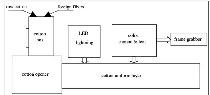
Figure 3. The image acquisition subsystem diagram (Ji et al. 2010)
