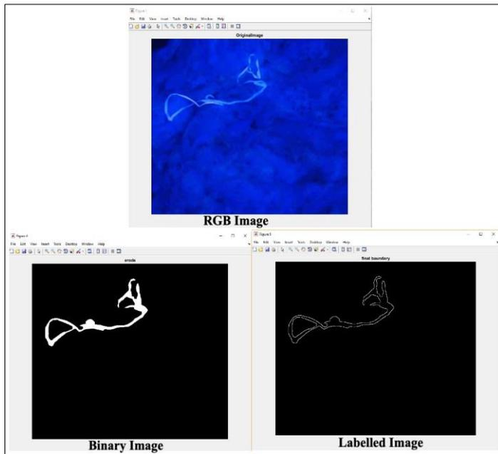
Figure 10. Detection of synthetic fiber in waste cotton bundle
