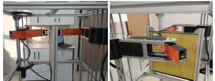
Figure 4. Robotic stitching of sandwich composites.
