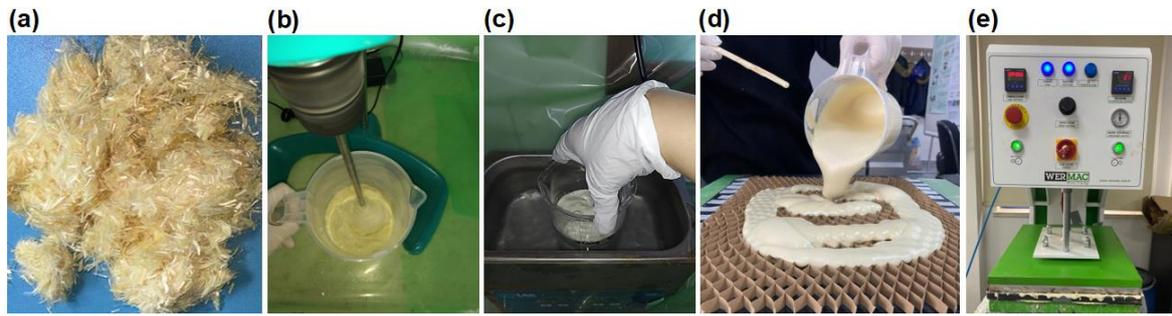
Figure 1. Core parts manufacturing stages; chopped Kevlar® fibers (a), mechanical stirring (b), ultrasonic stirring (c), molding (d), (e).
