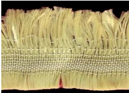
Figure 2. The waste selvage of the Kevlar® fabric.
