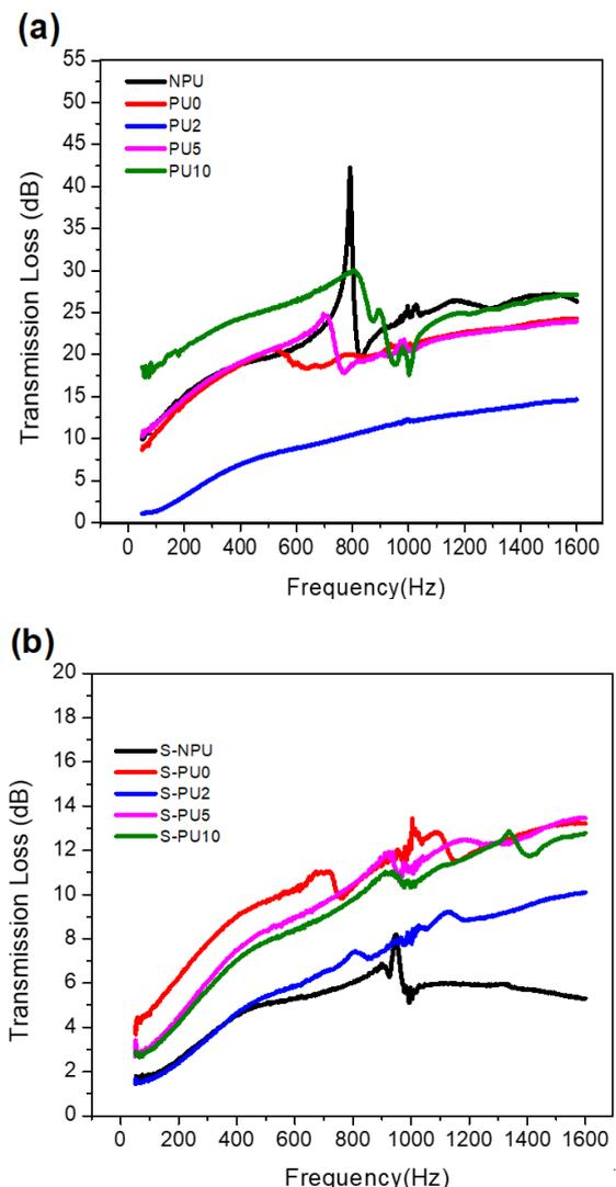
Figure 6. Sound transmission properties of unstitched (a) and stitched composites (b).
