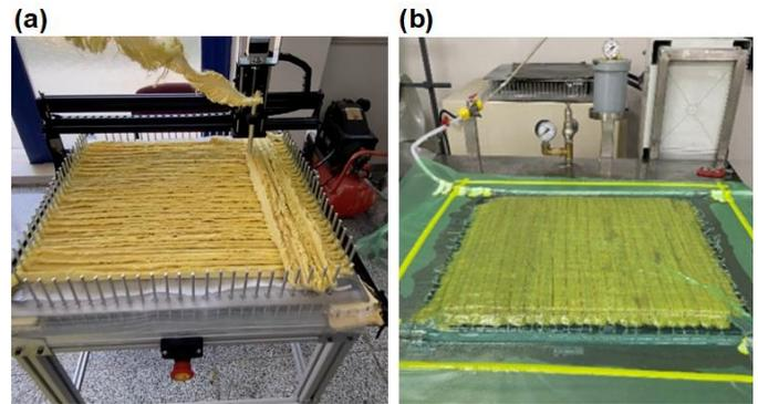
Figure 3. Fiber placement (a) and vacuum infusion (b) of sandwich composites.
