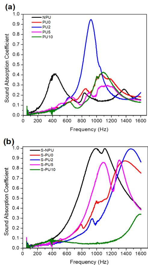
**Figure 5.** Sound absorption properties of unstitched (a) and stitched composites (b).
