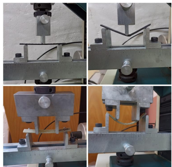
Figure 2. composite samples during 3 and 4-point bending tests
