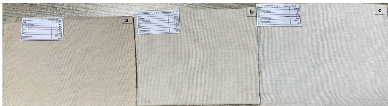
Figure 2. Samples dyed at a 3% shade using a) alum mordant, b) vinegar, and c) water only
